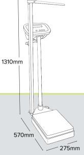
The elegant MUW ultrasonic scale calculates height, weight and BMI, with results displayed on the backlit LCD. This scale simplifies data collection and outputs user identification information without breaching confidentiality.
