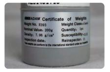
All weights meet requirements for testing to OIML standards
