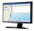
AdamDU quickly collects information from up to eight Adam balances simultaneously, via RS-232 or USB connections. An easy-to-use interface with a main command window lets users view and manage data capture sessions.
