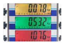
Display backlight changes colour during checkweighing
