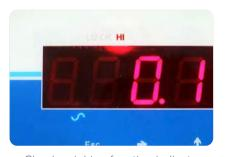
Checkweighing function indicator appears in three bright LED colours
