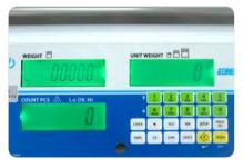
Backlit LCD displays show weight, unit weight and total count clearly
