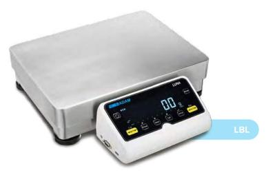
The Luna LBL combines the rugged durability of a heavy-duty base with the vivid, unmistakable clarity of the large, Luna-style weight display. LBLs are available in high capacities, while retaining a fine 0.1g readability.
